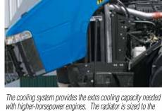
engine and can be accessed easily for cleaning.
